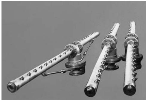
上水濾過池用、表面洗浄装置 Water Surface Cleaner for Use in Service Water Filtering Reservoir 口径・・・100A Caliber 流体・・・清水 Fluids: Clean Water 圧力・・・2kgf/cm 2 G Pressure 温度・・・常温 Temperature: Atmospheric temperature
